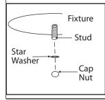
Tuck electrical wires into outlet box and position fixture over studs on mounting bracket assembly.
