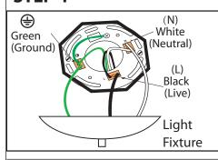
Connect (push) electrical wires from fixture into correct inserts.
